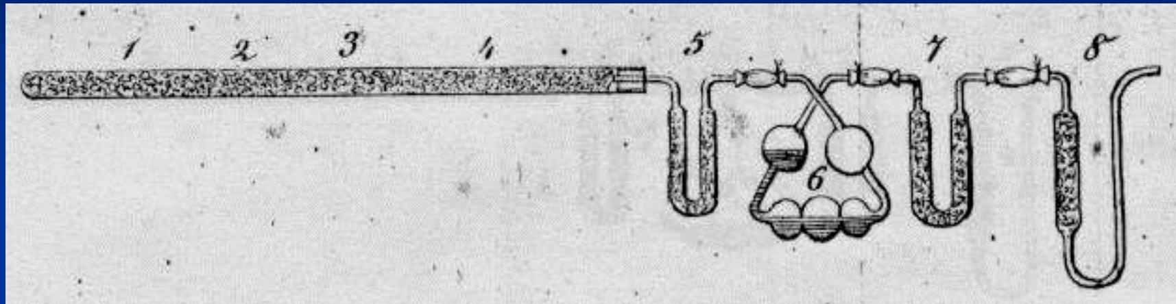
1. CuO and KClO<sub>3</sub>. When heated this mixture generates O<sub>2</sub> which carries the other gases through the apparatus. This obviates the necessity for breaking the tube at the end of the experiment.
